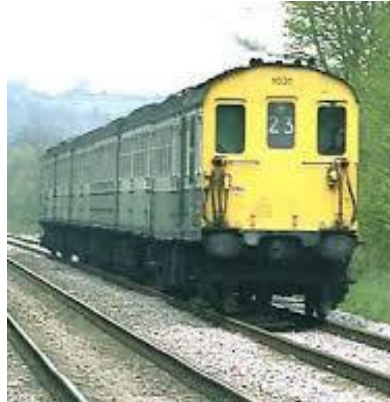
BR's 'Hastings' Units. These narrower trains were specifically built with flat sides to enable them to pass through the restricted tunnels south of Tonbridge
